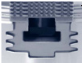
Patented multiple profile base jaw
