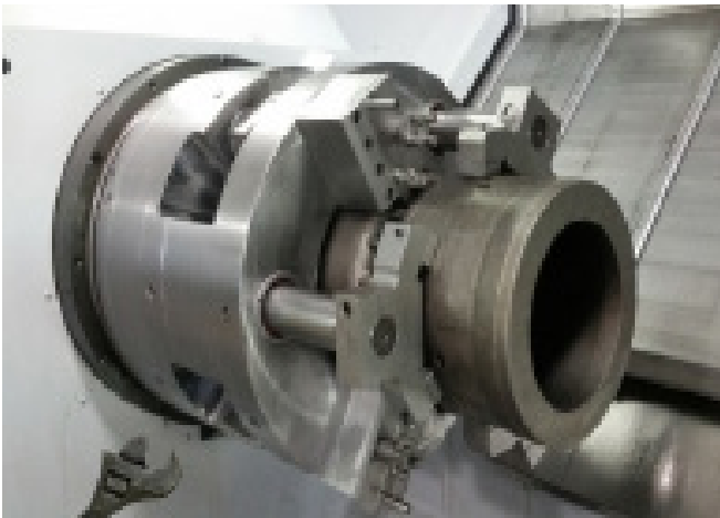
24" Hi-LO PC Chuck for Holding Locomotive Cylinder Liners
