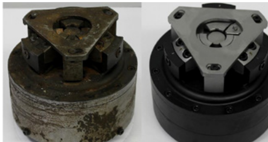
7" 3 Jaw Diaphragm Chuck Assembly with Special Tooling
