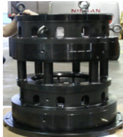
OD Grip Rim-Lok Collet Chuck for holding 14" Diameter Drum
