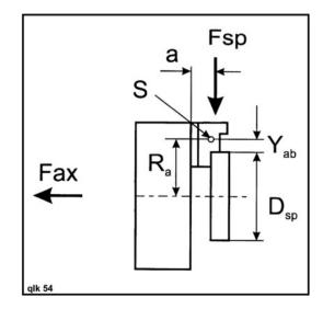
For the respective machining case, it must be checked whether the existing operating clamping force is sufficient.
