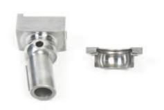
Also inspect the spherical portion of the actuator and the bearing race. If seizure is found on them, those surfaces would seem plated.
