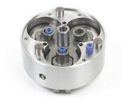
Left picture shows the back plate is removed from the chuck.
