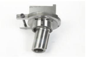
After setting, fix it by fixing bolt and remove from the vice.
