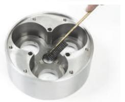
Spread high-adhesive grease on the actuator's sliding hole of the center of the housing.
